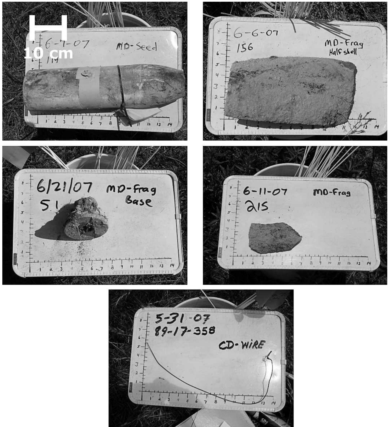
Figure 9. Representative items from Camp Sibert target classes. Clockwise from top left: 4.2" mortar (UXO class), partial mortar (Partial class), mortar fragment (OE class), cultural debris (Culture class), mortar base-plate (Base class).
