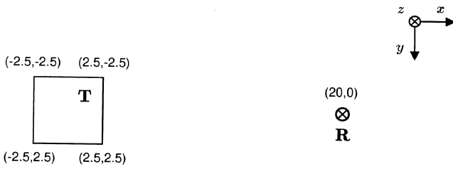
Figure 7. The transmitter–receiver geometry for the synthetic TEM data used as the first non-linear example. The origin is at the centre of the transmitter loop, and the coordinates are in metres. T and R indicate the transmitter and receiver, respectively, both of which lie on the surface of the model, that is in the plane z = 0 .
