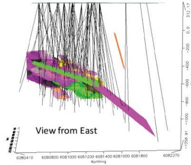
Figure 3. Plate modeling of the SQUID data for the deposit.
