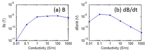
Figure 7. B and dB/dt responses for conductive half-spaces.
