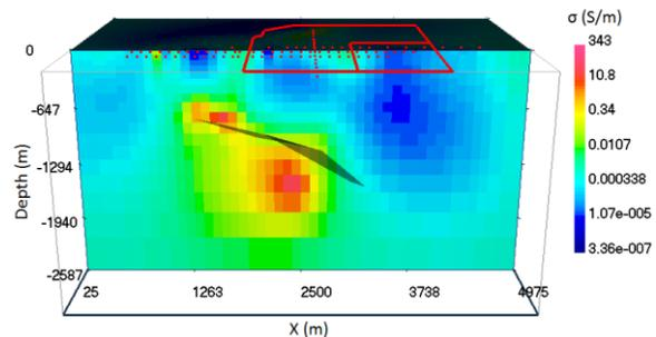
Figure 4. Conductivity model from the 3D inversion. The cross section on 5700N is shown. The plate models are indicated by the shaded surfaces.
