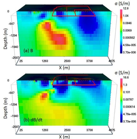
Figure 8. Conductivity models of the synthetic inversions using B-field and dB/dt data. The cross section on 5700N is shown.
