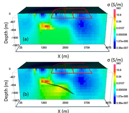
Figure 6. Conductivity models of the hypothesis test. The cross section on 5700N is shown. (a) The model with the deep conductor removed is used as the initial and reference model for the test inversion. (b) The result of the hypothesis test inversion. The plate models are shown as shaded area.
