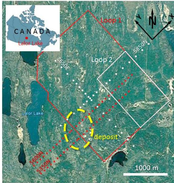
Figure 2. Layout of the SQUID TEM survey at Lalor Lake. Line 5350N and 5600N were collected with the transmitter Loop 1 (red) and Line 5850N and 2650E with the Loop2 (white).
