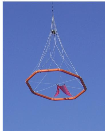
(c) Coil used to measure the vertical fields
